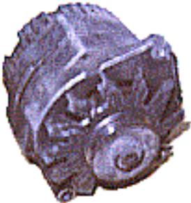
**The power source. A GM alternator (with built in voltage regulator).**
