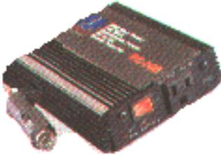
If a DC to AC power converter is added to the basic system, then a limited amount of 120 Volt AC power would also be available! DC to AC power converters electronically convert the 12 volt DC power to 60 hertz AC power at 120 volts. These boxes just connect to the battery on the generator, and provide AC power outlets for standard household AC power.
