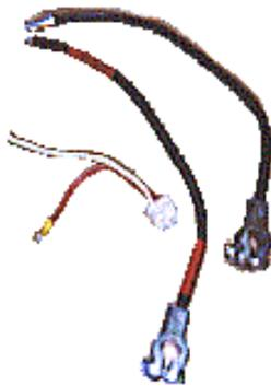
The small 2 wire plug shown was purchased at a local auto parts store for about \$3. This molded connector (with wires) is a replacement part for hooking into the two terminals (R, and F) on the alternator. It saved a bunch of time making two of the alternator connections and is well worth the cost. Your local parts store will carry something similar. The brand we bought was Calterm, Part number 08602.
