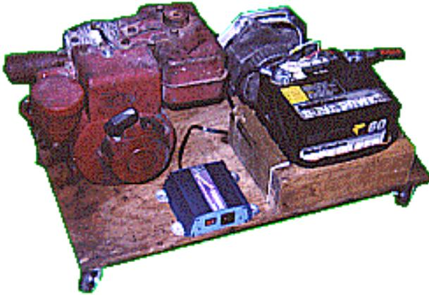
Provide at least 3" of space between the rear of the alternator and the battery. This will provide ample space for access to the alternator terminals. Next, use some scrap chunks of 2 by 4s positioned with the 2" side down, to build a 4" tall box around the battery. We cut them to length, and then secured them to the base from underneath using 2" wood screws.
