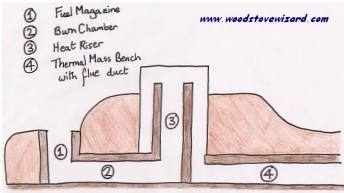
Fuel is loaded into the magazine (usually longer and thinner pieces than would normally be burnt) and fed into the combustion chamber. Air is drawn into the chamber past the fuel load and the ends of the sticks burn rapidly, usually with the characteristic roaring rocket sound. Combustion is rapid and hot to ensure maximum efficiency.
