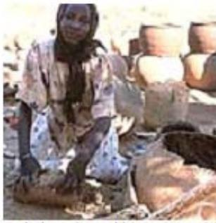
1. First, bowl-shaped moulds are created from mud and water – and left to dry in the sun. Clay is then pressed onto the moulds to form the desired size of pot. Clay rims and bases are added and the moulds are removed. The pots are left to dry in the sun.
