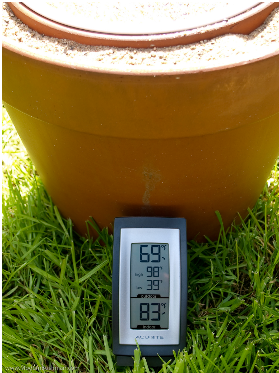
Thermometer reading 14° cooler inside the pot
